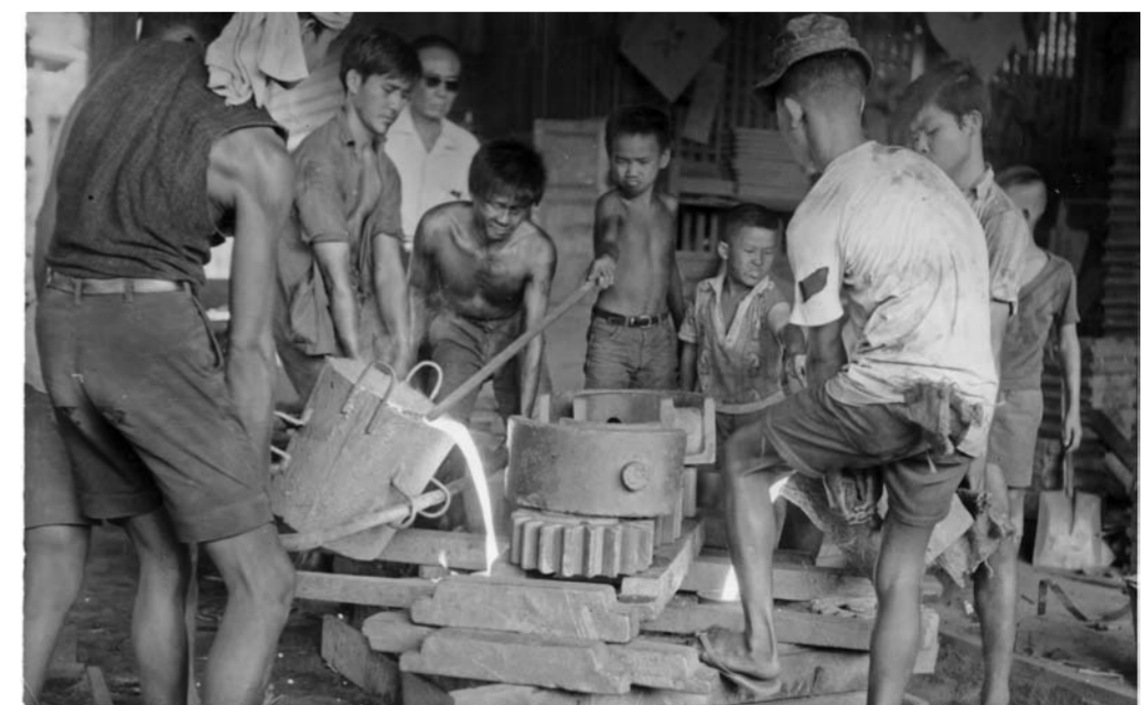
Iron foundry in Nakhorn Sawan, Thailand, Photographed by Robert Thomsen ca. 1970. The cupola furnace is tilted to tap out the iron.
