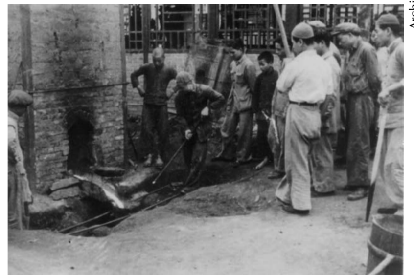
Operation of a cupola furnace in Chengdu, Sichuan, photographed by Joseph Needham in 1943.
