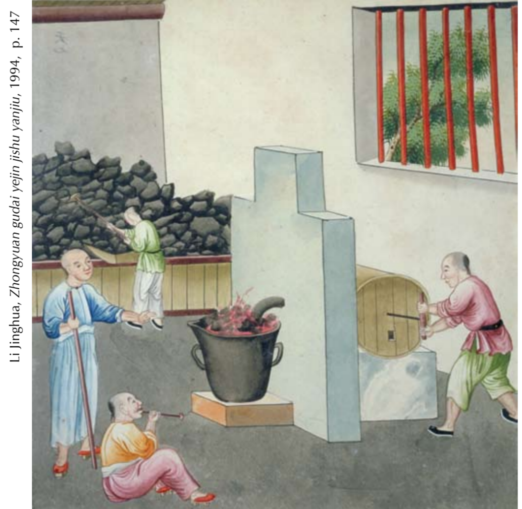
Chinese gouache painting, Guangzhou (Canton), 19th century. It is not clear what is happening here, but I suspect that iron is being melted in a crucible with the tuyère inserted into the mouth.
