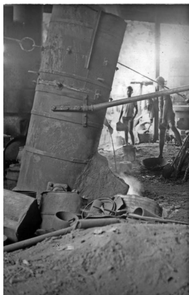
Iron foundry in Nakhorn Sawan, Thailand, Photographed by Robert Thomsen ca. 1970. The cupola furnace is tilted to tap out the iron.
